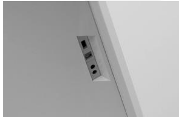
Embedded high resolution camera that can be used for barcode or QR code scanning
